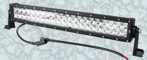
172102 - LED Fjernlygtebro 10-30V - 120W - 10800 lumen 628x111.2x86.5mm - IP 69K DT multistik - ECE R112
