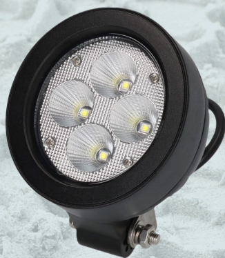
172269 - LED Arbejdslygte 10-30V - 40W - 4000 lumen 110x93x120mm - IP 68/69K Flood - ECE R10 - CISPR25 Class 3
